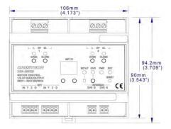
The DIN-4DIMFLV4 is a 4-channel lighting control module designed to support dimming of 4-wire 0-10 volt fluorescent dimming ballasts. A single model supports both 120 and 220-240 volt applications. Each channel handles up to 30 dimmable ballasts, and may also be used for switching of non-dimmable lighting loads up to 5 amps, as well as 1/2 HP motors.
